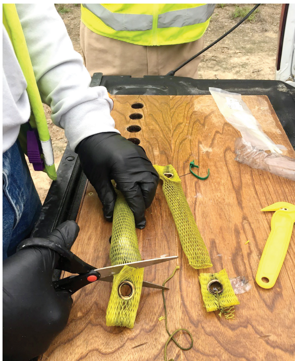
Preparing time-integrated groundwater sampler in deployment sleeve. (Photo Credit: GSI, Inc.)
