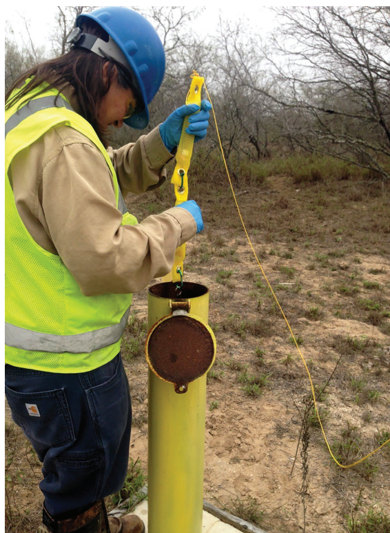
Deployment of time-integrated groundwater sampler in a monitoring well. (Photo Credit: GSI, Inc.)
