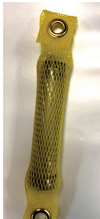
Time-integrated groundwater sampler. (Photo Credit: GSI, Inc.)
