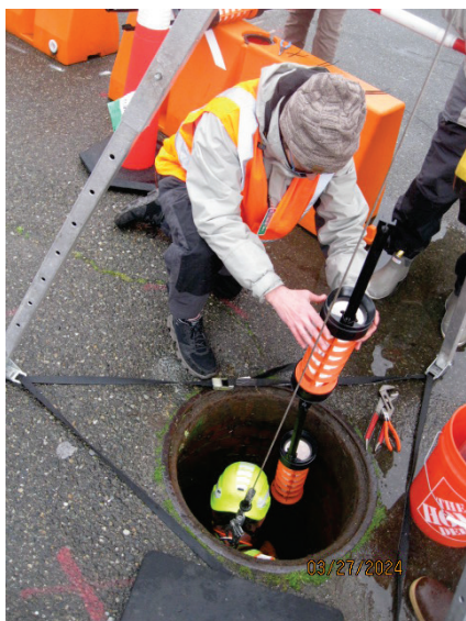
Deployment of I-Stub units within stormwater conveyance system at Puget Sound Naval Shipyard. (Photo credit: Brandon Swope)
