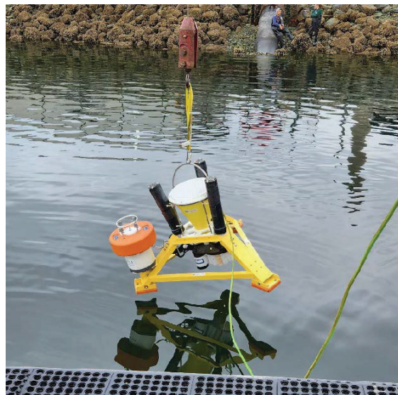
Deployment of the SABL adjacent to an outfall at PSNS for the duration of a storm season. (Photo credit: Molly Colvin)
