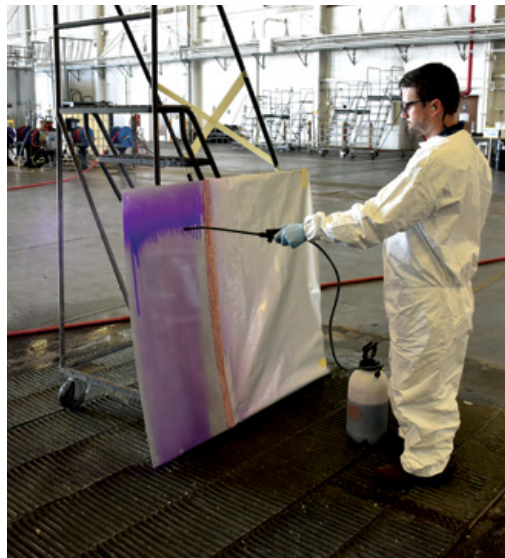
Spray application of eTCP ready-to-use at FRC Southeast to an aluminum panel. Production environment and panel orientation mimic spray conversion coating on aircraft as it is performed at FRC Southeast. (Photo Credit: Sjon Westre)
