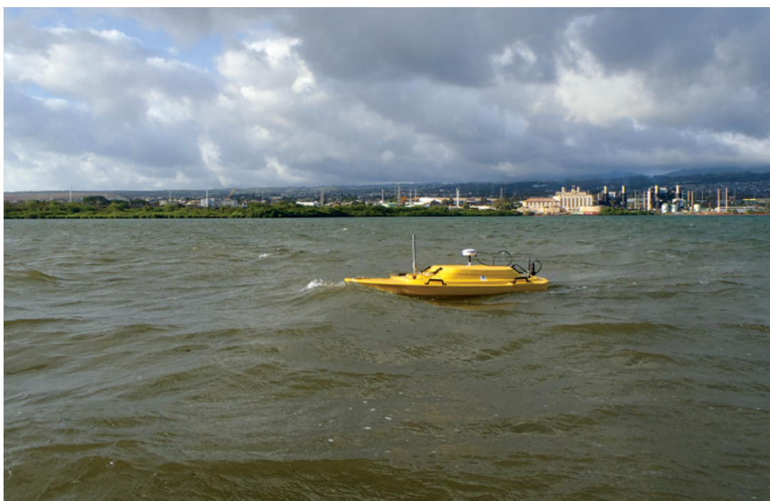
The NIWC “Z-boat” is key to this effort to develop a simple and cost-effective solution to ascertain the potential magnitude of recontamination occurring from unremediated underpier sediments slumping into dredged and/or remediated areas between piers. (Photo Credit: Chuck Katz)
