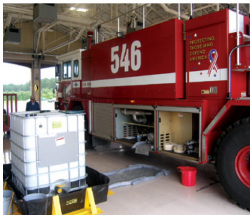
Pilot scale cleanout of a mobile Aircraft Rescue and Fire Fighting vehicle at NAS Meridian.
