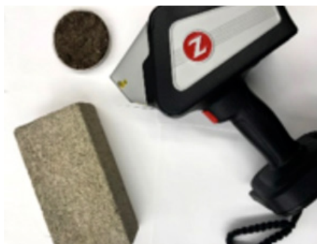
The LIBS analyzer will be used to measure contaminants on urban/industrial surfaces and within soils. (Photo Credit: Patrick Sims)
