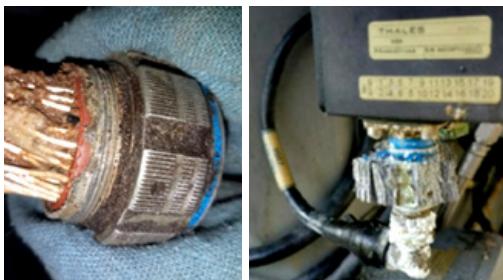
Degraded wires (left) and degraded connectors (right) from the V-22 Osprey Full Authority Digital Engine Control (FADEC) and Flight Control Wiring. (Photos compliments of NAWC-AD Patuxent River Wiring Laboratory.)
