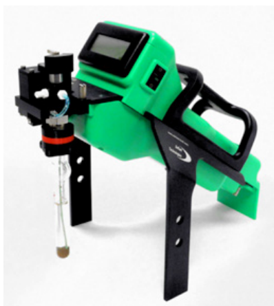
A number of COTS instruments including this one were demonstrated in this NESDI effort that sought to identify the most reliable device for the mobile analysis of indoor air and soil gas samples. (Photo Credit: Travis Lewis)
