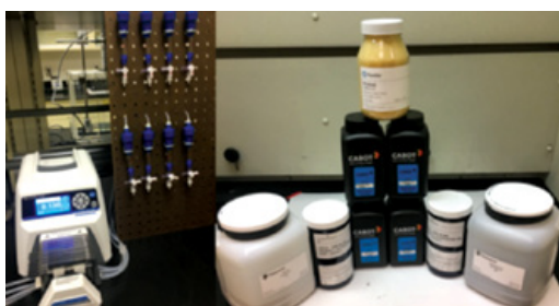
PFAS column treatability study construction at NAVFAC EXWC's environmental laboratory(left) and commercially available sorbents for batch and flow-through column studies (right). (Photo Credit: Jovan Popovic)
