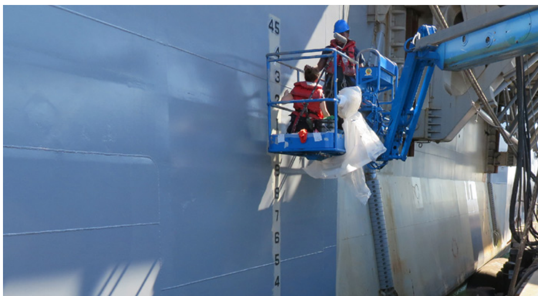
Sailors painting the freeboard of the USS Essex (LHD-2) with single-component polysiloxane topcoat.
