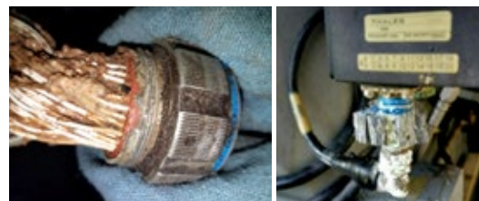
Degraded wires (left) and degraded connectors (right) from the V-22 Osprey Full Authority Digital Engine Control (FADEC) and Flight Control Wiring.
