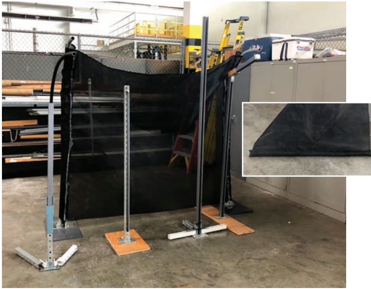
Itzel Godinez and her team completed the construction of prototype barrier designs including this one to prevent brown treesnake dispersal.
