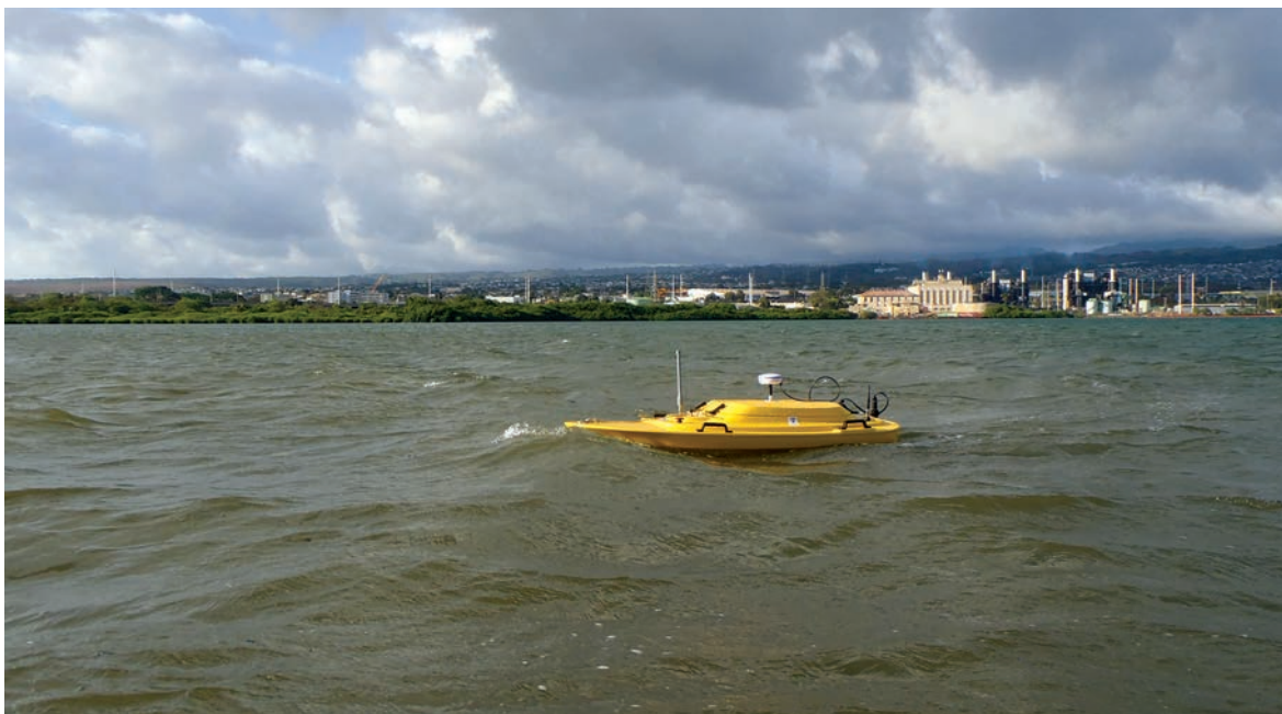
The NIWC "Z-boat" is key to this effort to develop a simple and cost-effective solution to ascertain the potential magnitude of recontamination occurring from unremediated underpier sediments slumping into dredged and/or remediated areas between piers. (Photo Credit: Chuck Katz)
