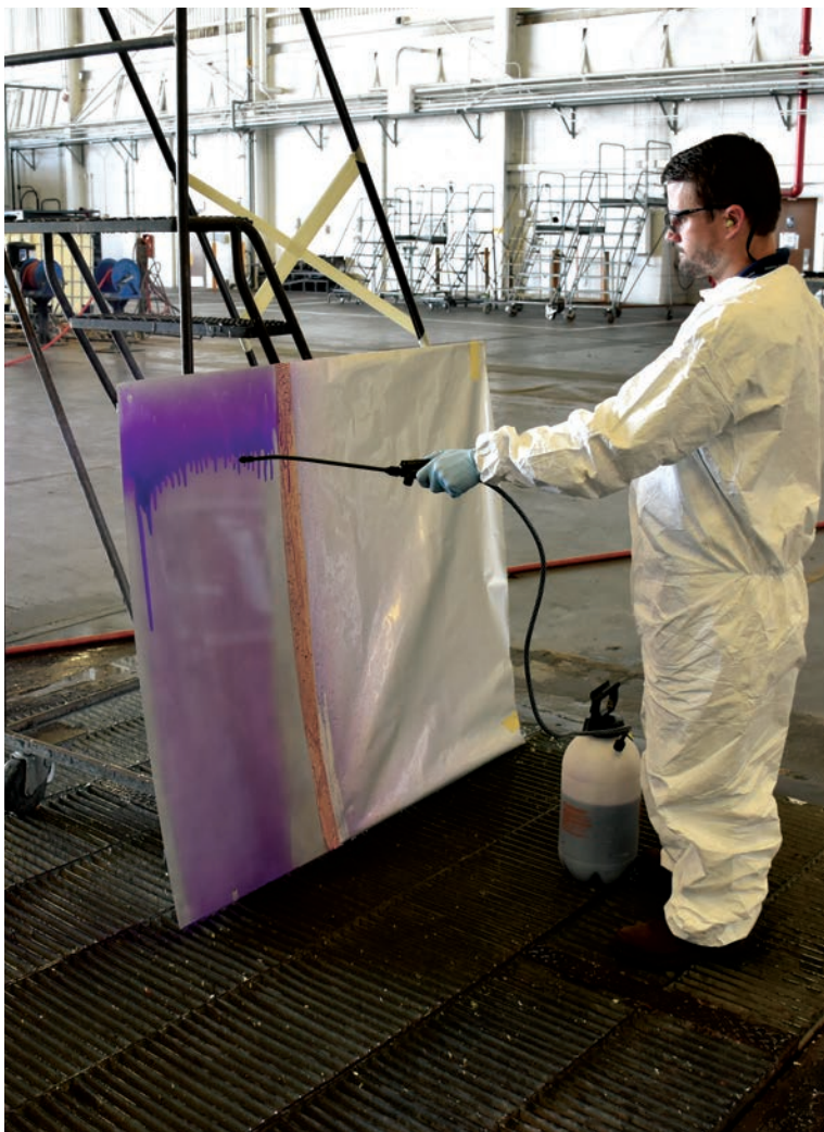
Spray application of eTCP ready-to-use at FRC Southeast to an aluminum panel. Production environment and panel orientation mimic spray conversion coating on aircraft as it is performed at FRC Southeast. (Photo Credit: Sjon Westre)
