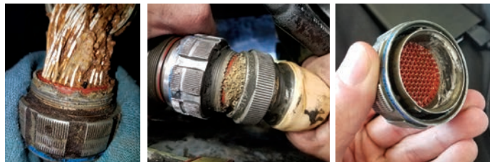
Degraded wires from the V-22 Osprey Full Authority Digital Engine Control (FADEC) and Flight Control Wiring.
