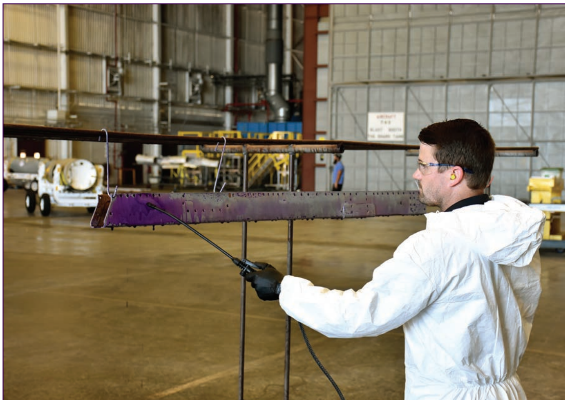
Peter Sheridan applies eTCP to aircraft missile launcher at FRC Southeast as part of this NESDI project's demonstration and validation. (Photo Credit: Joe Santa Maria)
