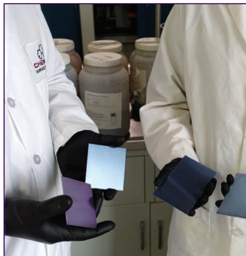
Comparison of dyed panels at the CHEMEON laboratory. Note the distinct color difference among the dyed panels. (Photo Credit: Sjon Westre)
