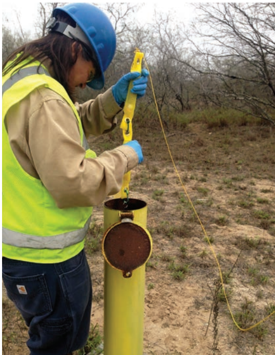
Deployment of time-integrated groundwater sampler in a monitoring well. (Photo Credit: GSI, Inc.)
