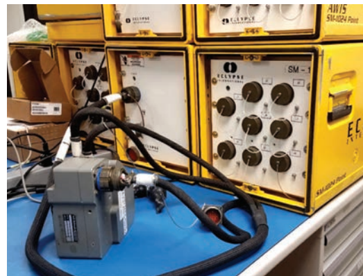
The V-22 Osprey Automated Wiring Test Set (AWTS) will act as the test bed for this NESDI project.
