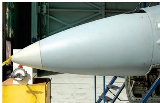
This NESDI project is studying the applicability of current laser depainting systems on composite nose radomes and other Navy aircraft components. Photo Credit: Steve Starnes
