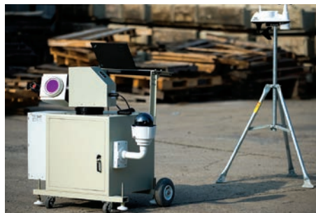
This opacity monitor is being demonstrated during this NESDI project. Photo Credit: Pat Morrow
