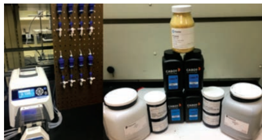
PFAS column treatability study construction at NAVFAC EXWC's environmental laboratory (left) and commercially available sorbents for batch and flow-through column studies (right).
