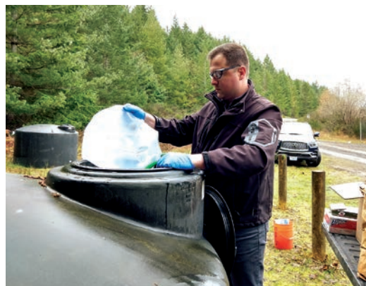
Preparing push with ^{13}\text{C} -, ^{15}\text{N} -RDX, conservative tracer and, in some wells, fructose.
