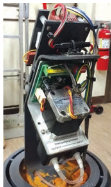
The PAWS system electronics and pump.
