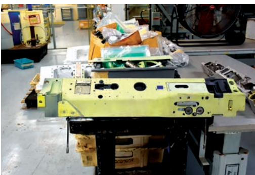
Investigators on this NESDI project are using a scrap Aircraft Armament Equipment part (a LAU-116 assembly structure and fairings) to demonstrate and validate an eTCP Violet spray application. Photo Credit: Joseph Santa Maria
