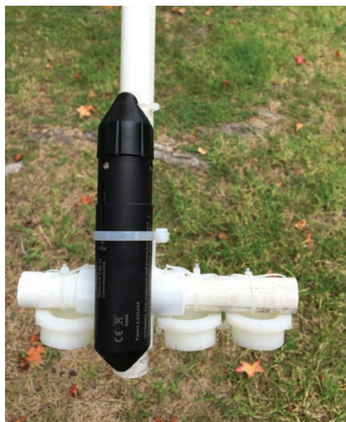
Prototype configuration of commercially available DGTs (round plastic sensors) for monitoring stormwater in end-of-pipe applications. Photo Credit: Gunther Rosen
