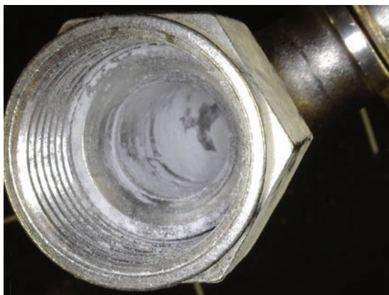
Fleet maintainers were unable to clean a contaminant (white substance) in aircraft oxygen lines with the currently-authorized Naval Oxygen Cleaner. Photo Credit: Kami Downey
