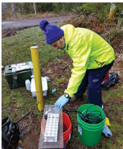
Post-push sampling for bacterial mineralization products.
