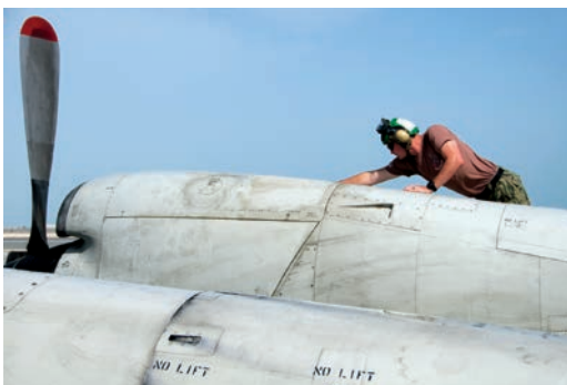
P-3 Orion components are being used in this NESDI project to assess the performance of hexavalent chromium-free adhesive bond primer.
