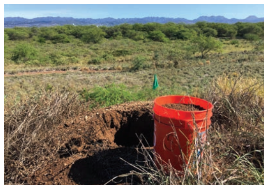
Sampling a dredged material stockpile for the demonstration of natural sediment EMNR at Pearl Harbor, HI. Photo Credit: Gunther Rosen
