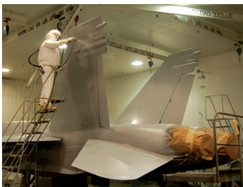
Worker applying polyurethane coating to an F/A-18 aircraft. Photo Credit: Jennifer Nunez
