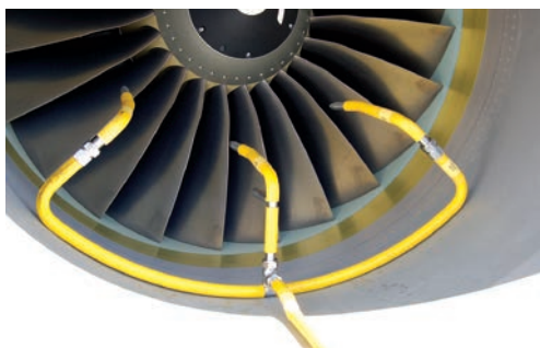
The EcoWash engine wash system nozzles in place during a test on one of FRC Southeast's flight lines. Photo Credit: Kami Downey
