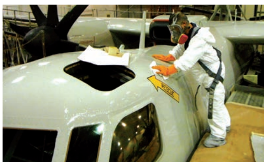
A Fleet maintainer applying a wipe solvent to an E-2 Hawkeye airborne early warning aircraft before the application of a primer. Photo Credit: Ed Lipnickas
