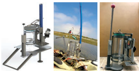
Left picture illustrates SUBS components. Middle picture shows the SUBS Sampler on a kayak in the open position. Right picture is the SUBS Sampler in the closed position.
