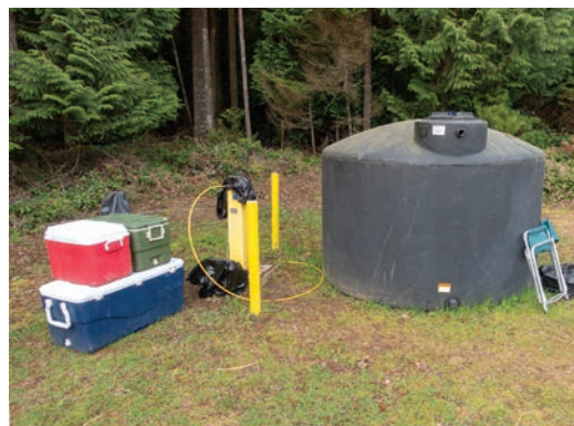
Push-pull test preparation with reservoir, in-well pump installed, coolers ready to ship samples.
