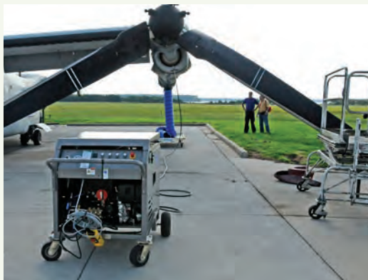
An H-53 engine wash demonstration was performed using the EcoPower small wash unit and effluent collecting kit. (Photo Credit: David Marriott)
