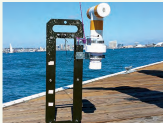
The prototype passive sampling device for sediment. (Photo Credit: Bart Chadwick)
