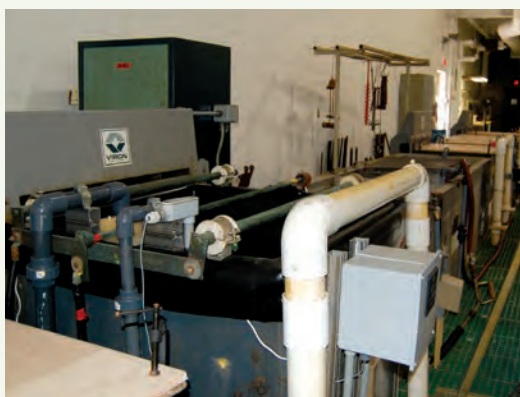
Process line designed for zinc-nickel electroplating. (Photo Credit: Ruben Prado)
