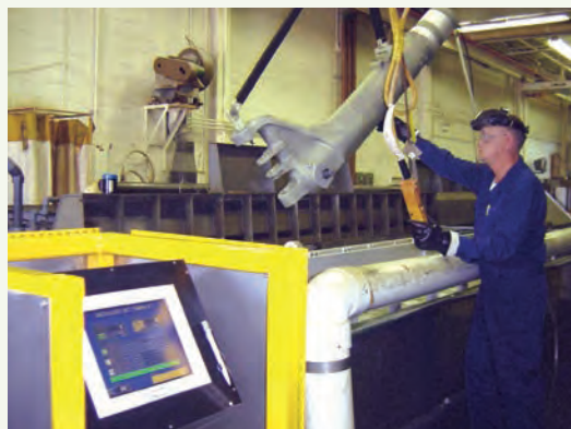
A shop artisan anodizing an EA-6B main landing gear in the modified anodizing tank at FRC Southeast. (Photo Credit: Ruben Prado)
