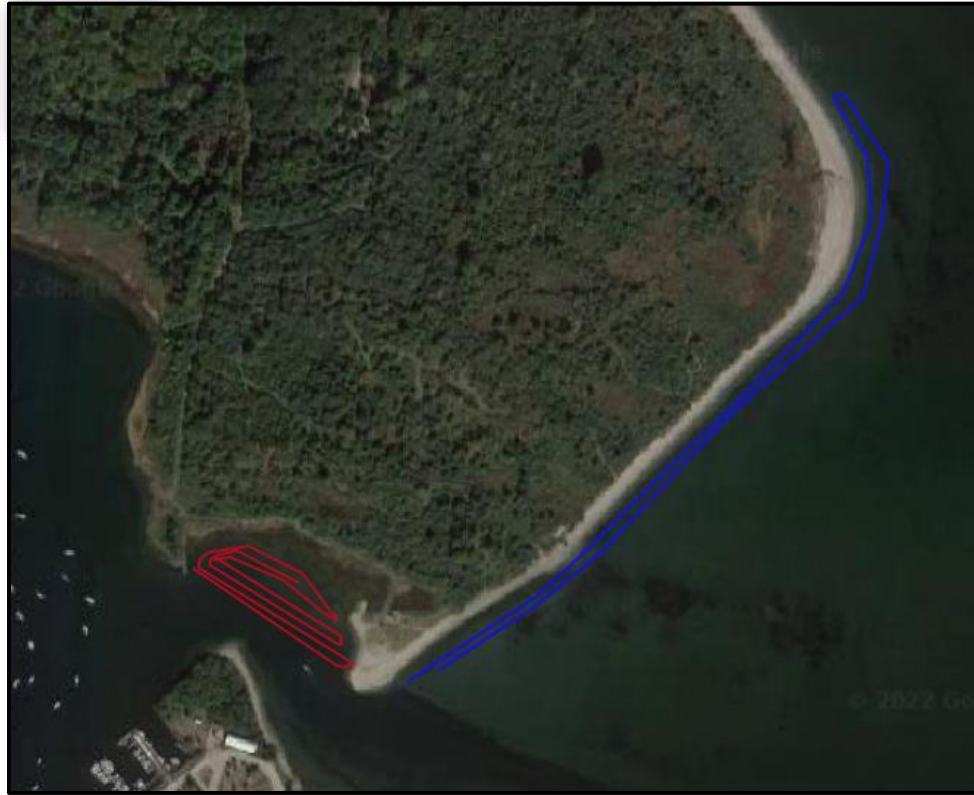
Figure 4. DTS cable installation near the Allen Harbor entrance channel (red) and along the Calf Pasture Point beach in Narragansett Bay (blue). These cables were connected around the south side of the sand spit, and each end was taken across the Allen Harbor channel to the interrogator instrument near the Quonset Hut visible near the bottom of the image. Connector cable segments not shown. (Source: SelkerMetrics).
