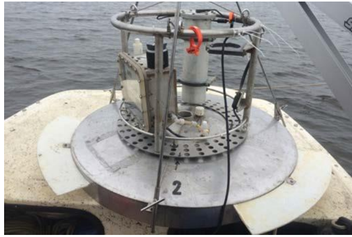
Figure 16. The UltraSeep system used to quantify groundwater seepage at the site in Allen Harbor in previous 2019 study (5). (Source: Reference 5).
