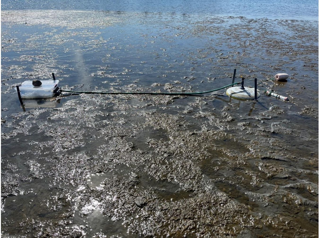
Figure 6. Example seepage dome, tube, and bag during low tide (Meter 3). The meters may not funnel seepage when exposed during low tides such as this. (Source: Anchor QEA).
