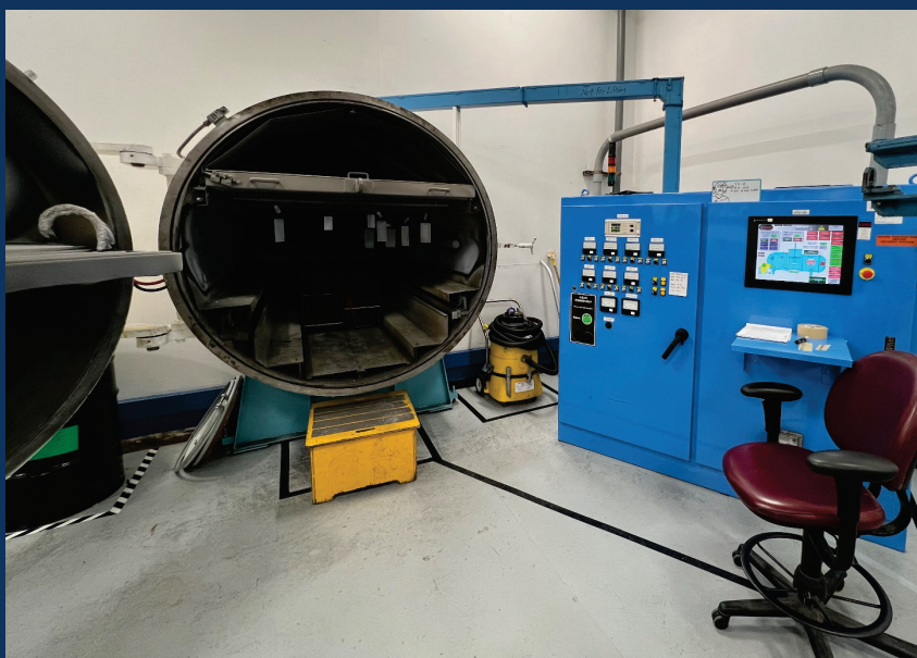
Supporting the Naval Aviation Enterprise, this Ion Vapor Deposition (IVD) vacuum chamber applies environmentally safe aluminum coatings onto critical components. This process is a key step in replacing carcinogenic hexavalent chromium post-treatments, ensuring the long-term health of our artisans while maintaining the high-performance corrosion resistance necessary for mission success. (NESDI Project # 634; Image Credit: Kaitlyn Elkins)
