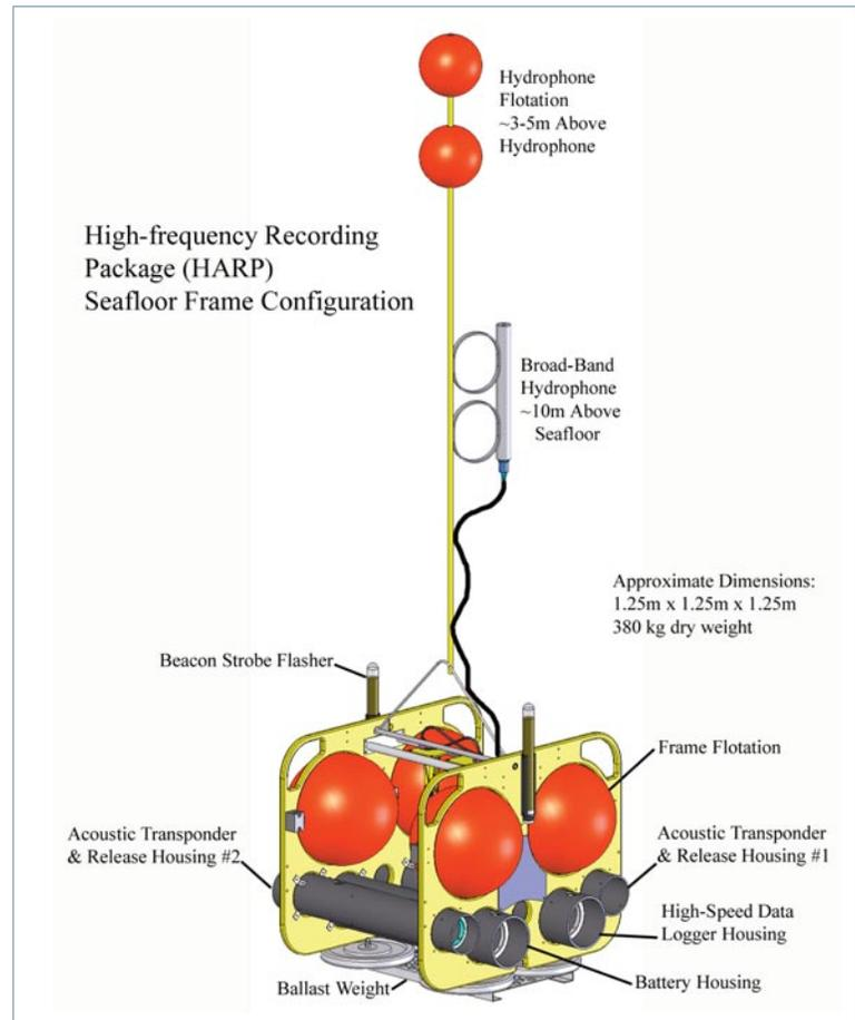
John Hildebrand, Sean Wiggins and colleagues at the Scripps Institution of Oceanography have developed the HARP for required Navy range acoustic monitoring. Under LMR program support, a new longer-lived, higher storage capacity HARP will be developed and demonstrated. New designs must stand up to challenging deep-sea conditions and not generate system noise that can interfere with recordings of animal sounds.
