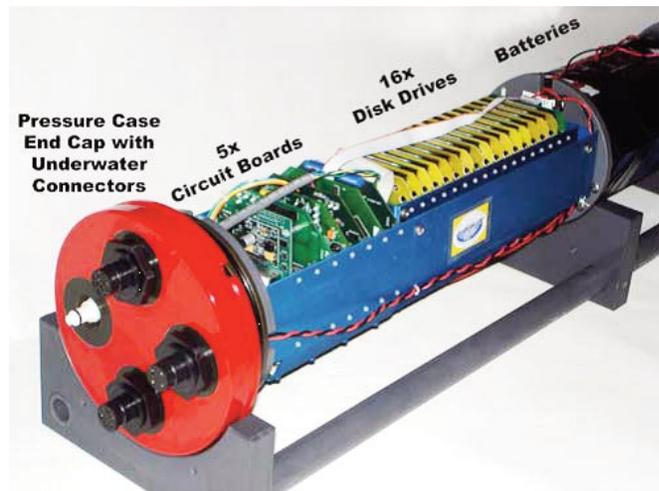
HARP data logger with underwater connectors.
