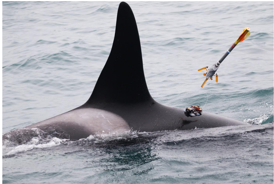
Mixed-DTAG+ successfully attached to a male killer whale in Iceland in July 2021, using the aerial remote tag system (ARTS).
