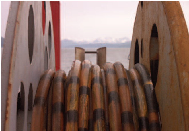
The towed hydrophone array, nicknamed Delphinus, was developed by TNO for the detection and classification of marine mammal vocalizations, as well as to localize marine mammals in real time.
