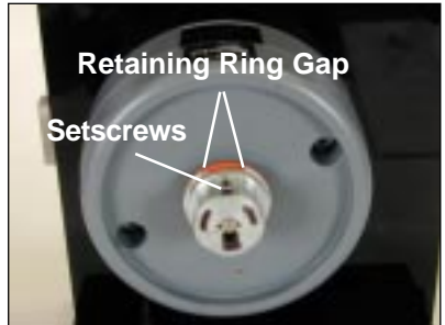
Figure 29 - Align Retaining Ring
