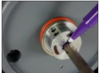
Figure 21 - Mark Spindle Flush to Hub
