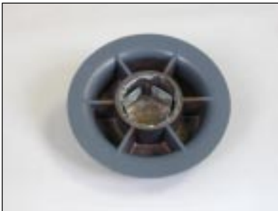
Figure 30 - 5-Sided Flat Spring in Dial
