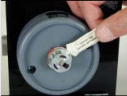
Figure 27 - Apply Lubricant to Ret. Ring
