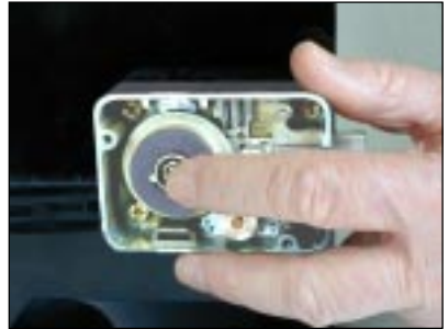
Figure 25 - Maintain Pressure on Spindle Assembly
