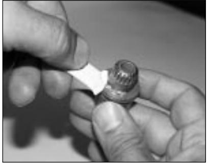
Figure 23 - Apply Lubricant to Hub
