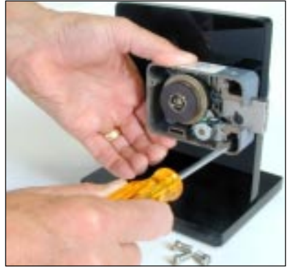
Figure 6 - Tighten Mounting Screws
