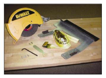
The saw consists of a heavy-duty metal chop saw attached to a modified aluminum base and uses a 12-inch abrasive metal cutoff blade. The Cabinet Bolt Saw carriage is hinged and spring loaded making it easier to control the cut and safer to operate.
