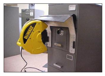
to the container, the saw can slide to the proper position to cut the hardened bolts.
