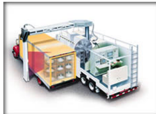
Figure 2-17. MobileSearch™ system in action, scanning truckload of TV monitors.
