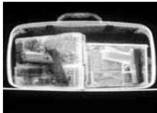
Figure 2-22. Backscatter image of "boombox" with 2 concealed pistols, 1 traditional and 1 plastic Glock 17.
