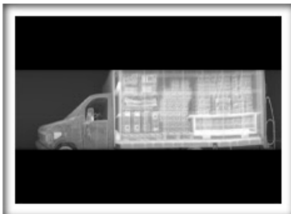
Figure 2-20. Backscatter image of van carrying power supplies and rifles.
