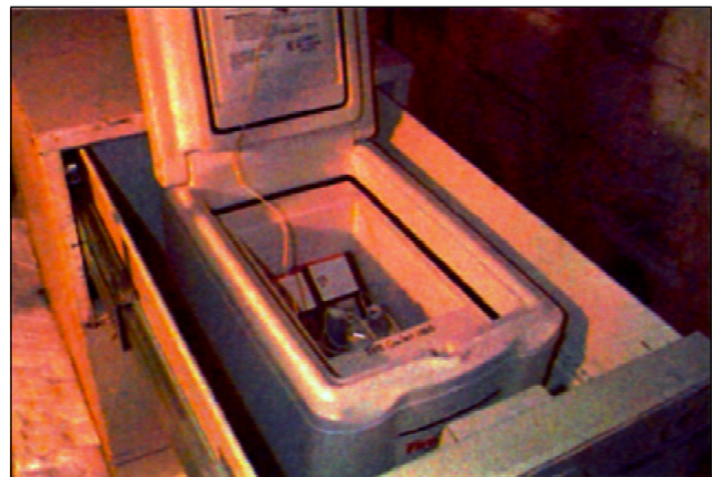
Figure 1. Fire Cooler 1000 inside security cabinet.
