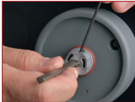
Figure 7. Tightening Hub onto Spindle Using Allen Wrench
