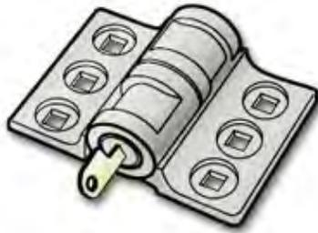
Figure 8-2.--TUFLOC Door Lock
