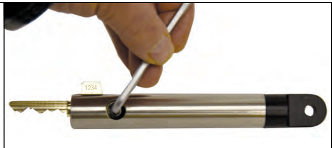
Figure 6-2.2. Remove Hex Head Screw
