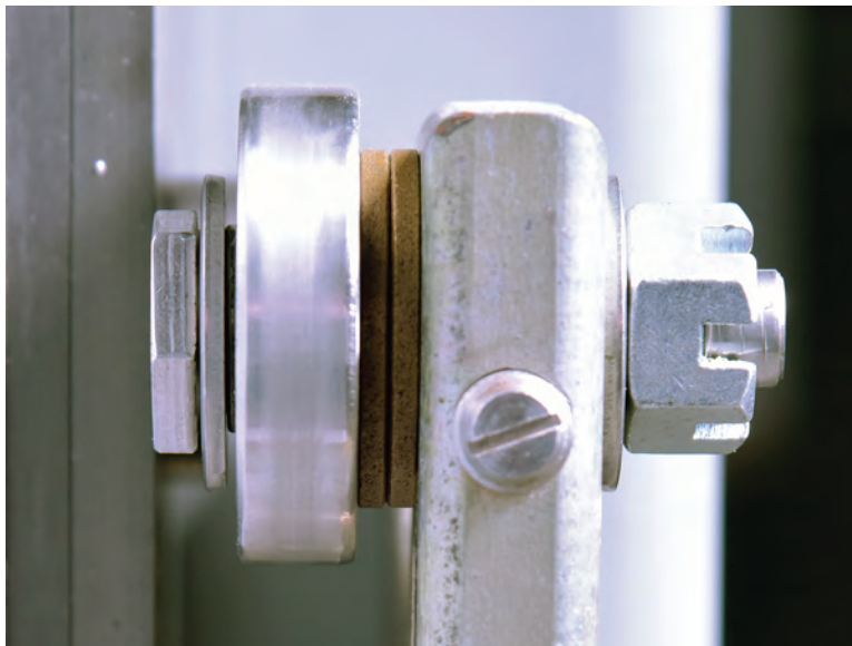
Figure 5-3. Orientation of Bolt, Thrust Bearings, & Washers
