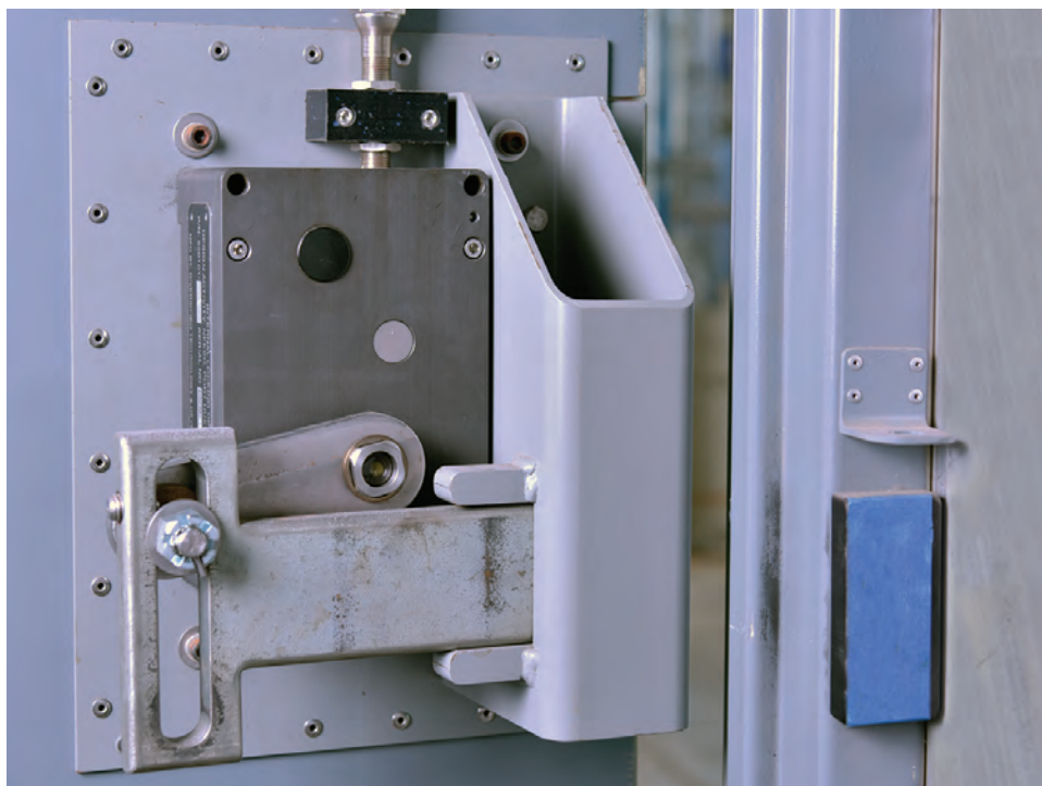
Figure 5-9. Reassembled Personnel Door Sliding Boltwork
