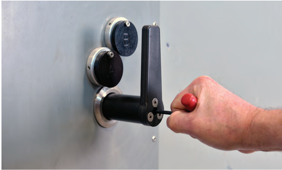
Figure 5-4. Removal of ILD Handle
