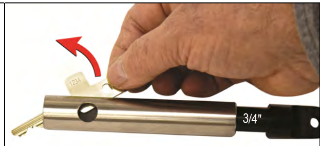
Figure 6-2.3. Slide Key Guide Core Away From Key Guide Shroud and Remove Key
