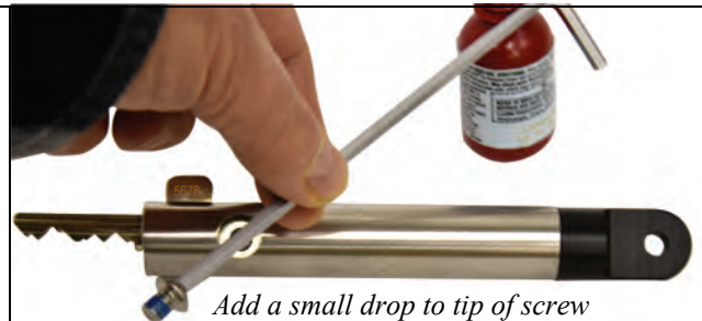
Figure 6-2.6. Prepare Hex Head Screw for Reinstallation
