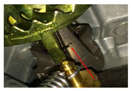
This is the incorrect position of the detent sprint where the lower leg of the detent spring has slipped off the worm wheel pin and rests against the slide block. Notice space between the spring leg and the worm gear wheel pin.
