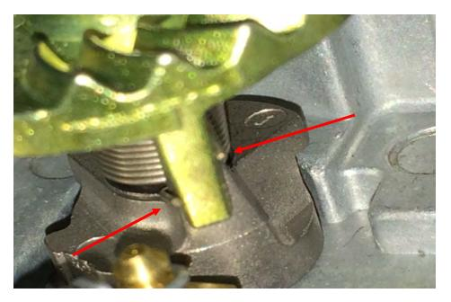
This is the correct position of the detent spring with a leg on either side of the worm wheel pin and the slide block. Notice spring legs resting against opposite sides of worm wheel pin.
